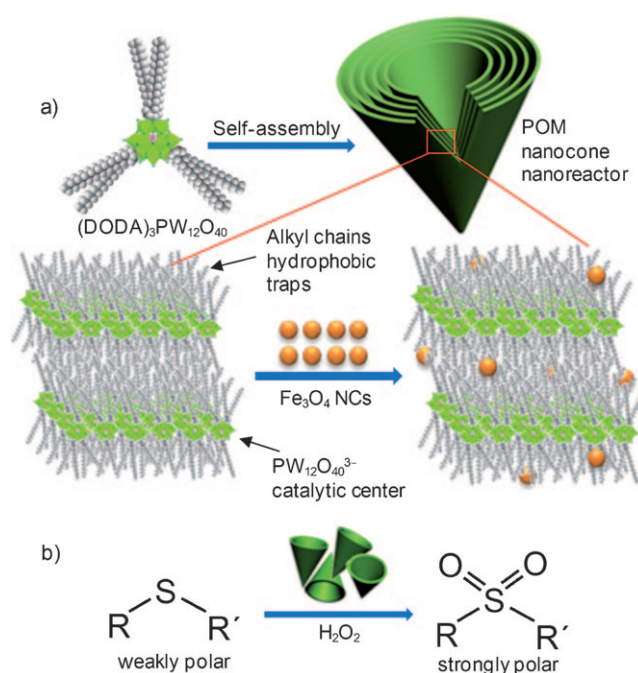
Figure 1. a) Schematic illustration of a POM nanocone nanoreactor. b) Oxidation of sulfides to sulfones in the presence of the cones as a catalyst.
